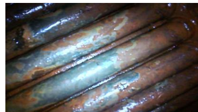
Fig 3b: 21 days after DCI Treatment-shell side
