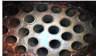
Fig 2b: 9 days after DCI Treatment-tube side
