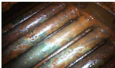
Fig 3a: Before DCI Treatment-shell side
