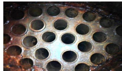
Fig 2b: 9 days after DCI Treatment-tube side
