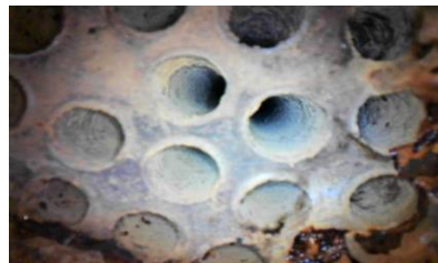
Fig 2a: Before DCI Treatment-tube side
