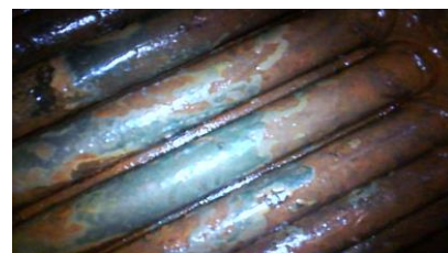
Fig 3b: 21 days after DCI Treatment-shell side
